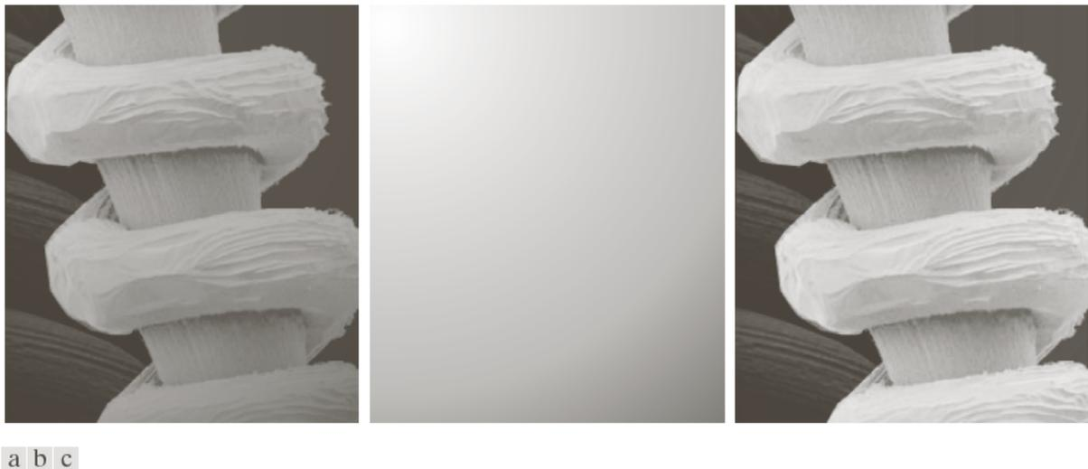
**FIGURE 2.29** Shading correction. (a) Shaded SEM image of a tungsten filament and support, magnified approximately 130 times. (b) The shading pattern. (c) Product of (a) by the reciprocal of (b). (Original image courtesy of Mr. Michael Shaffer, Department of Geological Sciences, University of Oregon, Eugene.)
