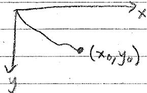
+ With  $\dot{y}$  pointed down, the speed is  $\sqrt{2gy}$ , so the time to travel length  $dl$  is  $dl/\sqrt{2gy}$ .
