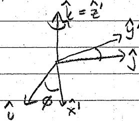
+ Next rotate by  $\theta$  around  $\hat{x}'$  to align principal axes with  $\hat{x}=\hat{x}'$ ,  $\hat{y}$ ,  $\hat{z}$  axes
