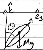
+ Gravity exerts a torque  $\vec{\tau} = (R\hat{e}_3) \times (-Mg\hat{e}_1) = MgR\sin\theta \hat{x}$  which is along the line of nodes (always). It will cause  $\hat{e}_3$  to precess around  $\hat{e}_1$  (if the top is already spinning around  $\hat{e}_3$ )
