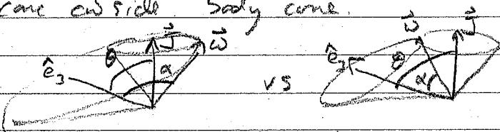
+ The wobble rate (angular velocity of precession of  $\hat{e}_3$  around  $\hat{J}$ ) is  $\dot{\psi}$  by the definition of the Euler angle.
