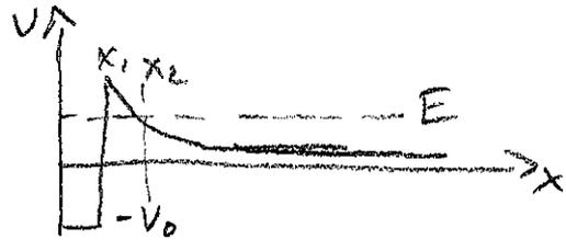
+ Each time it hits edge of box, it has a chance to tunnel. That's once every  $2x_1/v$  for speed  $v = \sqrt{\frac{2}{m}(E+V_0)}$
