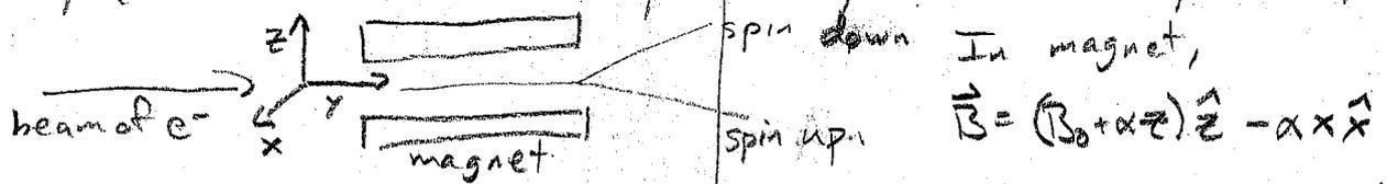
1) The  $x$ -component is needed for Maxwell's eqns but unimportant b/c Larmor precession averages it away for large  $B_0$
