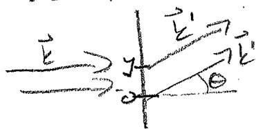
Light from different parts of the screen with the same  $k'$  go off to a far away detector at  $\vec{r}$  at the same angle  $\theta$ .
