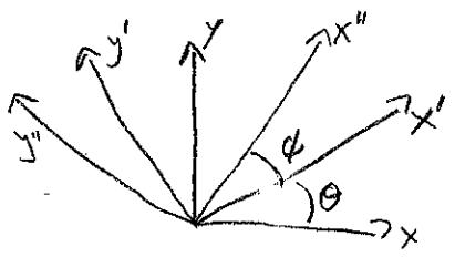
As you can see from the figure, rotations are composed by adding the angles
